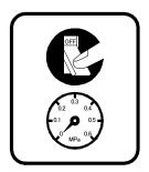
Be sure to cut the power and air supply off before adjusting or maintaining the machine. Otherwise, you may suffer electric shocks or may be entangled in the machine.
