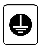
Be sure to provide grounding of the third class or better for installation.
